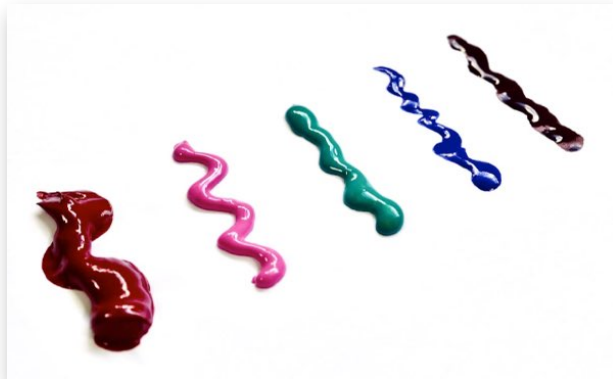
Several types of acrylic paint, from left: Heavy Body, Soft Body, Fluid, High Flow, Acrylic Ink
